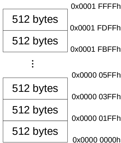
SC32F11xx7 series 128 Kbytes APROM sector partition diagram
