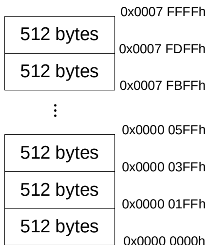
SC32F11xx9 series 512 Kbytes Flash ROM sector partition diagram
